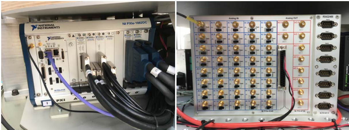
Figure 5.2: National Instruments™ Real Time PXI System [left] including its analog I/O (female SMA connectors) and serial RS-485/RS-422 (male D-sub connectors) interface board [right].
