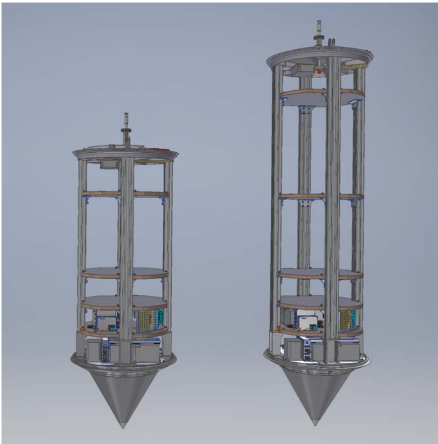
Figure 4.1: Drop tower capsule versions equally equipped with the Standard Capsule Equipment (SCE). [left] Standard Capsule for drop, catapult, and GraviTower operation. [right] Long Drop Capsule.
