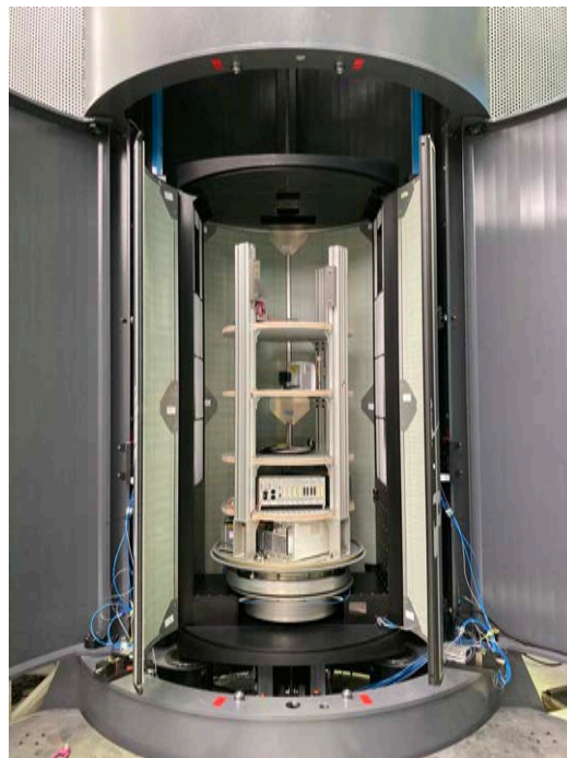
Figure 2.9: View inside GraviTower's open slider - with Standard Capsule on RCM.
