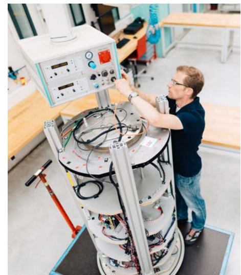
Figure 2.6: EGSE-to-capsule interface unit.
